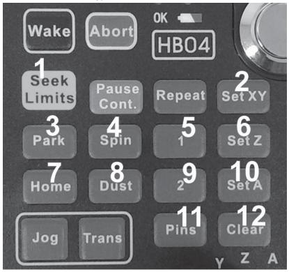
The large numbers (1 - 12) represent the codes to add to the scanon and scanoff variables in the CNCSCRN.INI file. Here is an example:
