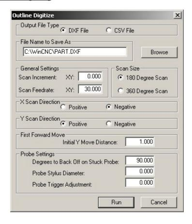
WinCNC supports simple X/Y only outline/edge digitizing. This is part of the Up/Down/Side scan feature and must be enabled by the machine manufacturer (or Microsystems World CNC) before it can work.
