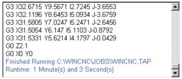
The message display window is the main output window displaying the commands that have been executed, messages to the user, or errors that have occurred during an operation.
