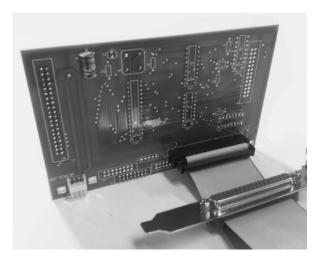
Below is the PCI-7200 card on the left, the Daughter Board on the right and the spacer/screw assembly. Note the matching holes in the corners of the Daughter Board and the PCI-7200 card. There is another set in the other end of the cards as well, just beyond the ribbon cable connector.
